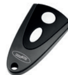
Handsender Micro-Novotron 512 2-Kanal, 433 MHz, KeeLoq-Wechselcode
